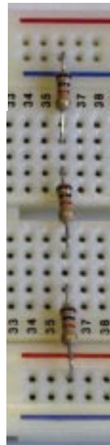
Photo.1.7. Three resistors connected in series on the breadboard.
