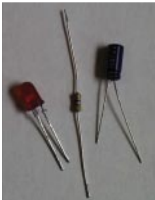
Photo.1.3. Left to right: Light-emitting diode, resistor, electrolytic capacitor.
