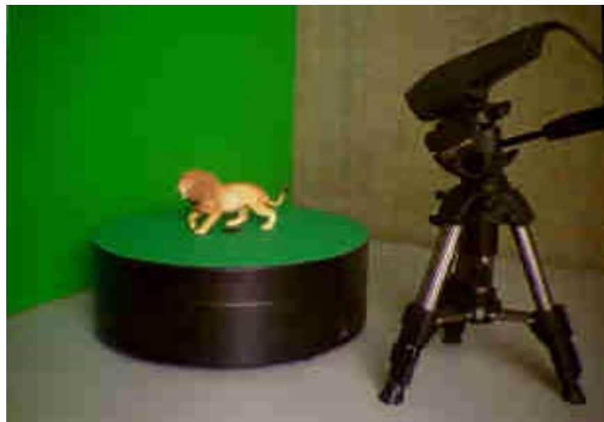
Fig.1. A computer-controlled turntable and a Video camera are used to scan an object.
